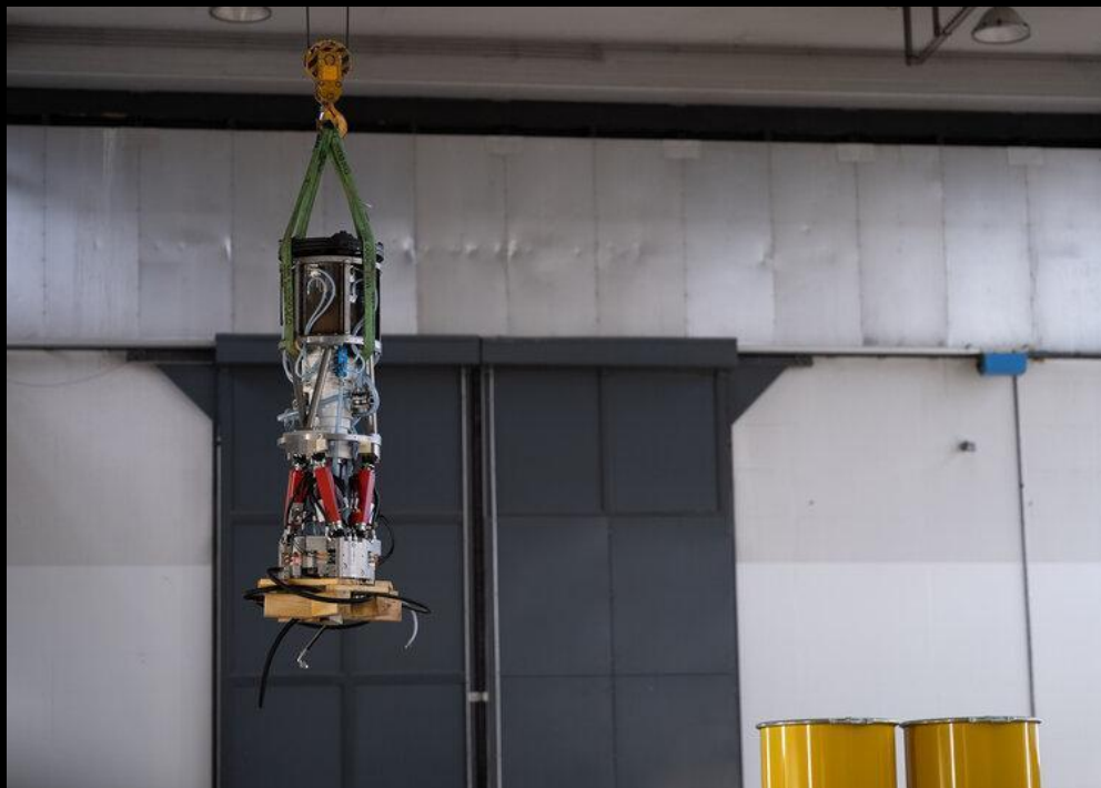
Erosion and Steering subsystem being transported using our 25 t crane
